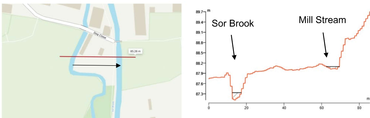
Figure 8 - Elevation of the Sor Brook in comparison to the Mill Leat. (Source: DEFRA 2025)
